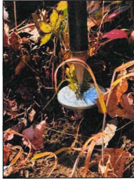
The rebar with Vermillion County Surveyor Cap
